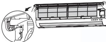
When removing the air inlet panel for internal cleaning or others, open the grill and then pull it to this side.
