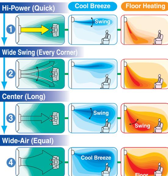
Thanks to automatic control of air flow volume and air flow direction, comfortable air conditioning of the entire room can be done effectively.
