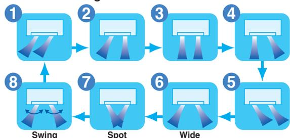
The airflow direction from the right and left louvers can be controlled individually. Eight different air flow patterns can be selected.
