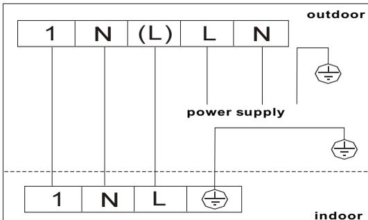
*Note: For some models the wires has been connected to the main PCB of indoor unit by manufacturer without terminal block.*
