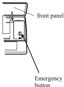
The emergency button is located on E-box cover of the unit under the front panel.
