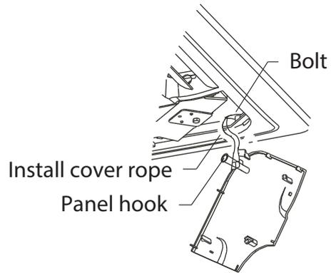
Re-installed into the style grid.
