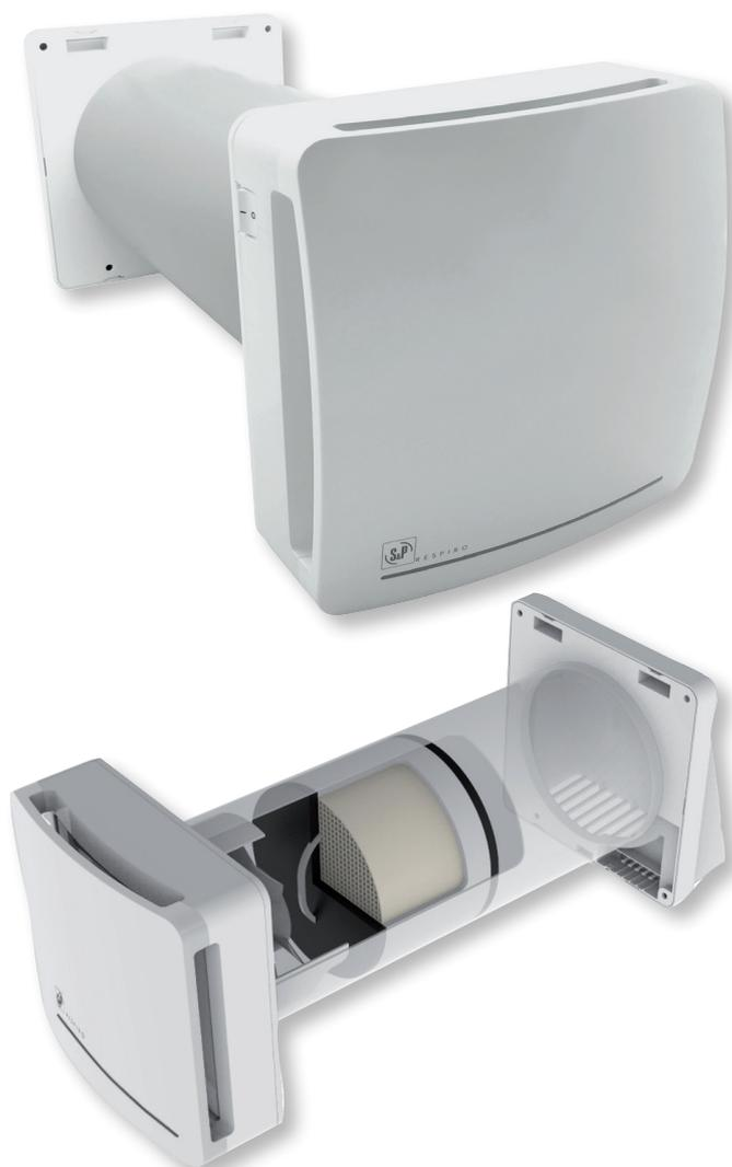
Decentralized ventilation unit, with heat recovery, for single rooms in domestic or commercial applications. Elegant design that allows its adaptation to any environment. Brushless motor with low consumption electronic control. Ventilation system through an reversing motor and a heat exchanger with a performance up to 93%. Designed for a continuous operation, the unit adjusts the airflow proportionally to the humidity level (model RD), ensuring excellent indoor air quality.
