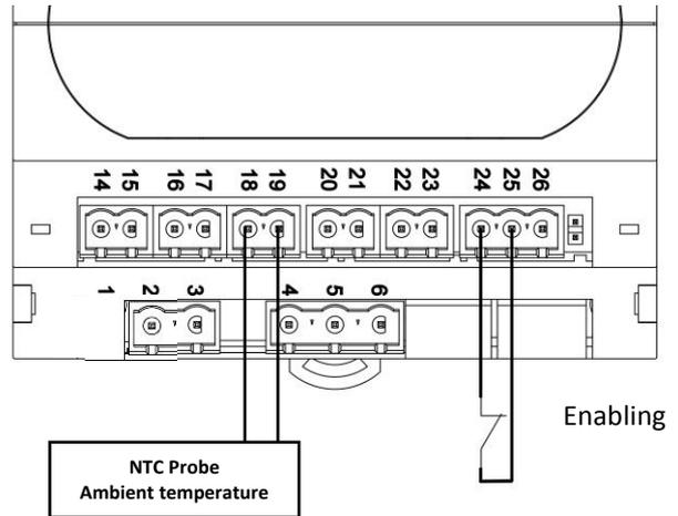
In this mode, it is possible to set the two configurable outputs (Do4 and Do5) to manage a few typical functions of a sauna or Turkish bath, like the supply of essence, the managing of inlet or outlet fans.
