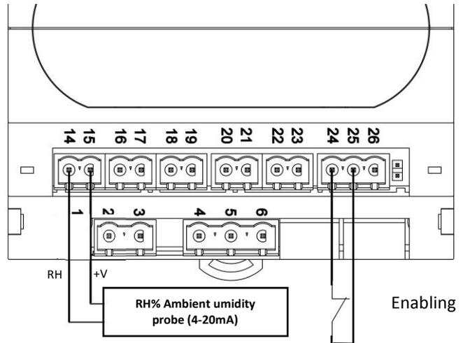
The Bp proportional band is the percentage value of the humidity around the set point; within this value the humidifier works proportionally. Example: if the proportional band is set on default value 10% (-5% / +5% set point value) and humidity is set at 50%, below 45% the humidifier will work at 100% of steam output; above 55%, the humidifier will not produce steam. Between 45% and 55%, the humidifier will optimally regulate steam output.
