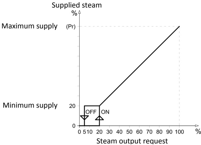
described in chap. 2.4. The minimum steam supply is fixed at 20% and is managed with an activation hysteresis; the maximum supply had in correspondence with a maximum requested output, corresponds to the percentage set in the first level variable (Pr). If, for example, on an ES6 producing 6Kg/h of Pr steam 100% is set, maximum supply will be 6Kg/h; but if Pr is reduced to 50%, maximum supply will be 3Kg/h.
